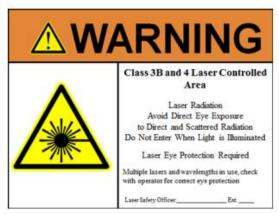
Unattended Laser in Operation, Class 3B or Class 4 must be identified with warning sign when the exterior boundry of a non-interlocked laser use area that contains unattended open beams is in operation. Example:
