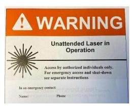
Temporary Laser Controlled Areas for Class 3B and Class 4 laser systems must have appropriate NOTICE signs. Example:
